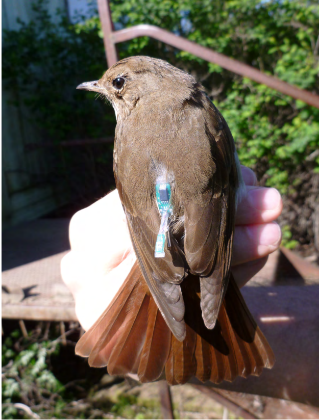
Figure 1. Hermit Thrush wearing Migrate Technology Ltd model P65C2J13 light-level geolocator, attached with Stretch Magic® leg harness.
